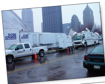
Figure 1.33 Production truck (far left), graphics truck and two satellite uplink trucks stitched together along with backup power generator for NCAA basketball.
