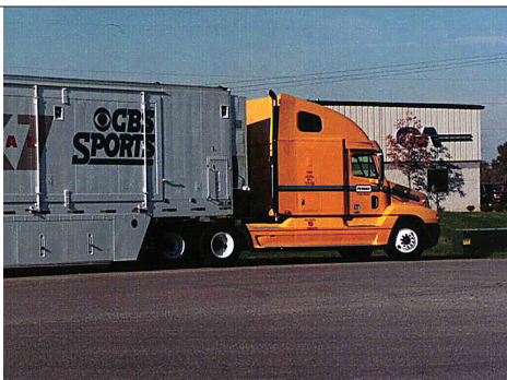
Figure 1.9 NMT's DX7. NMT has the largest fleet of remote trucks (43) in the world. This truck is typical of the latest generation of high-end standard-definition trucks. It has a digital infrastructure (NMT uses the DX prefix to signify a standard-definition digital unit), and can support up to 16 cameras and record and playback 16 sources at the same time. This unit has CBS livery on it as CBS uses the unit on a regular basis. (Source: Gerling & Associates)
