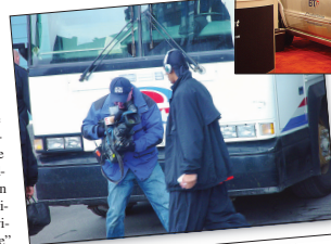
Figure 1.16 Contemporary camcorder in use by a "one-man-band" photographer. Front half is a professional camera, at the rear is a component VTR.
