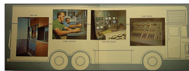
Figure 1.3 Graphic that depicts remote truck basic operations in terms of early 1960s gear
