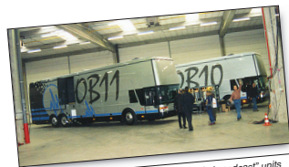
Figure 1.2 Two Belgium remote, or "outside broadcast" units built on a VAN HOOL T 927 two-level coach. Each unit is essentially a television production facility on wheels. Each can switch up to 30 cameras into an integrated television program. (Source: Allacam)
