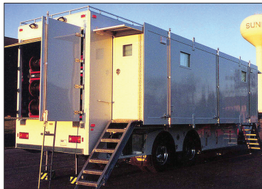
Figure 1.10 Many units today have sides that expand out once the trailer is parked. These are known as expandos. There are units that expand out both sides, known as double expandos. Some even expand out the back, thus triple expandos. Although the required equipment has gotten smaller over time, the complexities of today's production vs. your father's requires much more equipment and many more people in the trailer. These expandable sides allow for more "people" space. (Source: Gerling & Associates)
