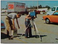
Figure 1.12 1970s version of EFP. The professional television camera was just becoming truly portable but, as this photo demonstrates, they were still 10 years from incorporating high quality videotape recorders (VTRs) into them. The camera, center, feeds video to the VTR on the left.
