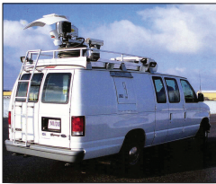
Figure 1.13 Modern ENG truck, mask and microwave antenna on top of truck extend upwards to about 40 feet. (Source: Gerling & Associates)
