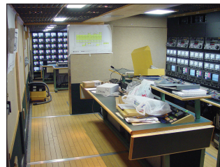
Figure 1.25 Television production trailer under construction. When parked with the sides expanded, the interior space can be as much as a large mobile home. Far monitor wall is for the production compartment, monitors to the right are for the tape area.
